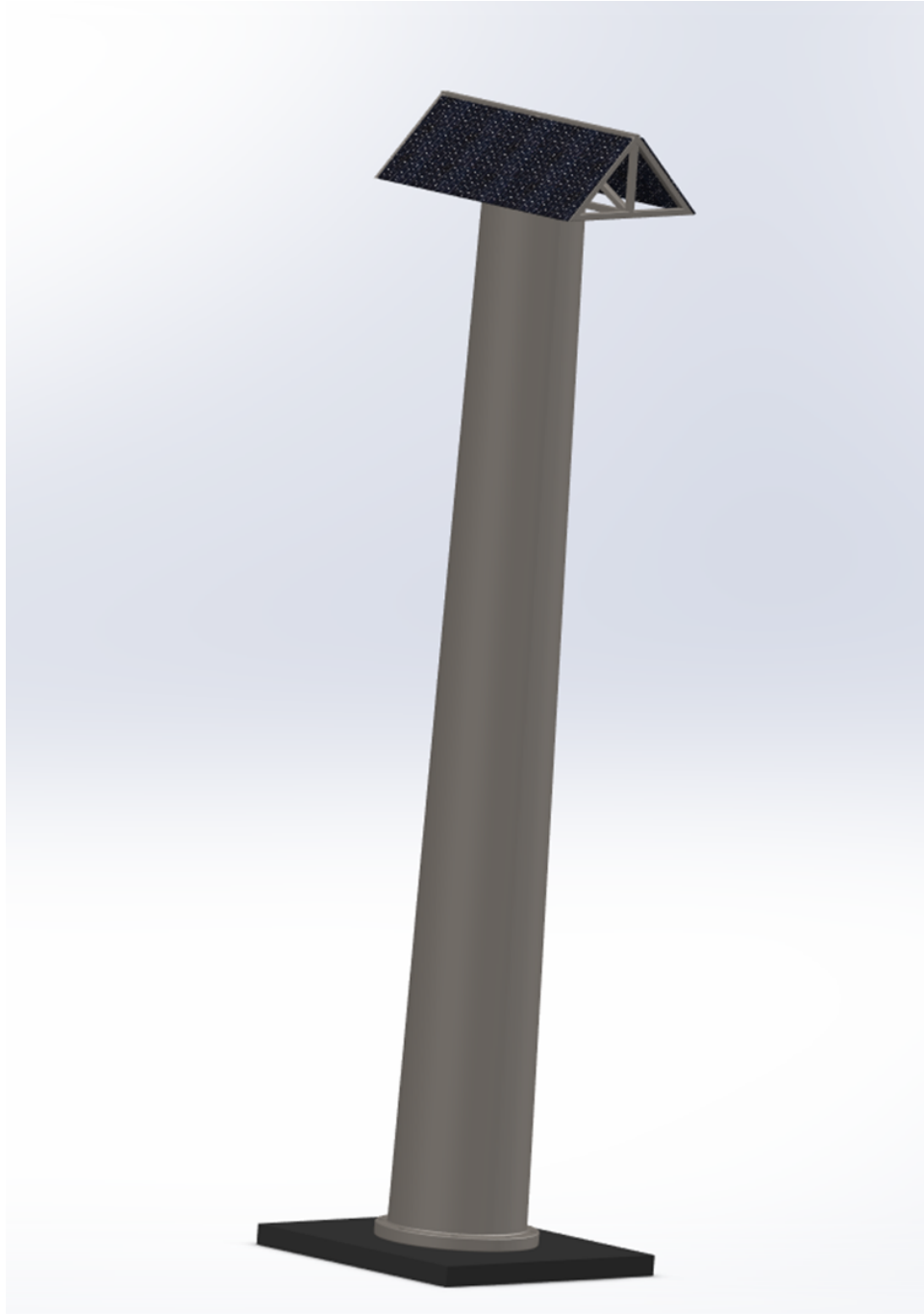
Figure 2: Tower, horizontal structure, and top solar panels modeled for the wind simulation.
